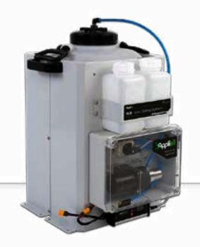
Tank size is 25 L. It can be removed for cleaning or better mixing. There is a hose quick coupling on the lid. The hose is removed by pressing the blue ring. It is the only applicator in the world, that has an insulated wall to protect the bacteria from high temperatures. If the bacterial liquid temperature is more than 40 degrees, there is a risk of degrading the bacteria.
